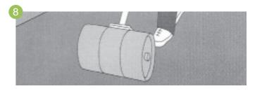
When the floor has been completely covered re-roll the area again to maintain good adhesive contact.
