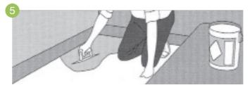
Fold the sheet half way back taking care not to disturb the positioning of the flooring. Apply the recommended adhesive onto the subfloor using the application techniques recommended by the manufacturer, from the wall to within 20cm of the guide line. Replace the carpet carefully and accurately back into position and roll with a 68kg flooring roller to ensure overall contact with the adhesive. Repeat for the other half of the sheet.
