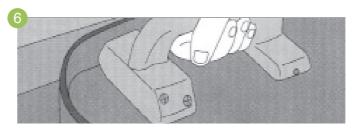
Using an Araseur or a sharp knife trim the carpet to fit against the perimeter walls. .
