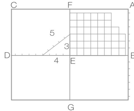
Lay out tiles along one wall to leave at least half a tile border along both walls. Measure the distance AB to give the border plus a number of whole tiles.
